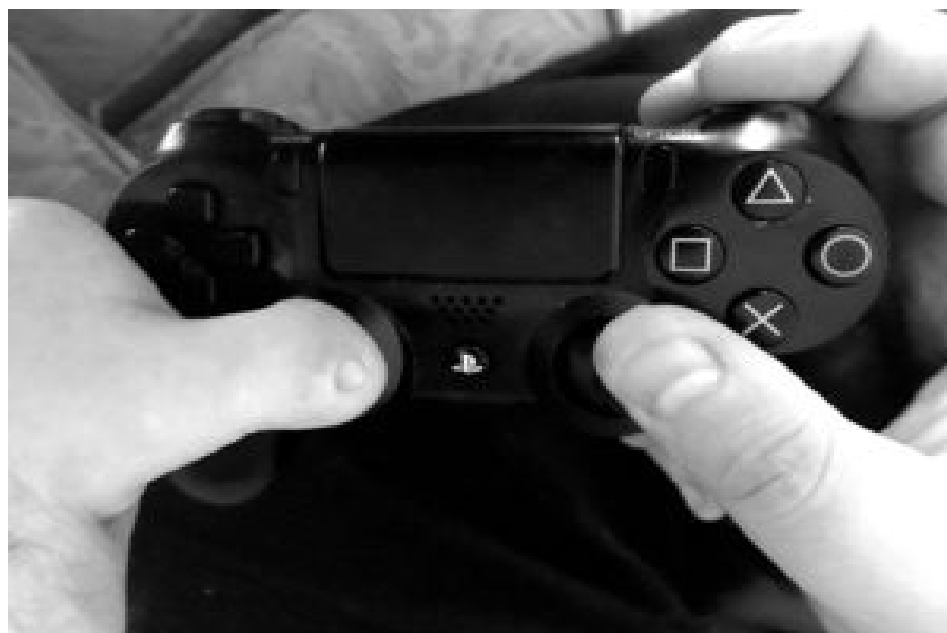
Figure 2 – The current interaction style of the author: left thumb at elbow joint operates left analogue stick and D-Pad, right hand operates right analogue stick and all buttons. Photo: Mathew Dagleish
