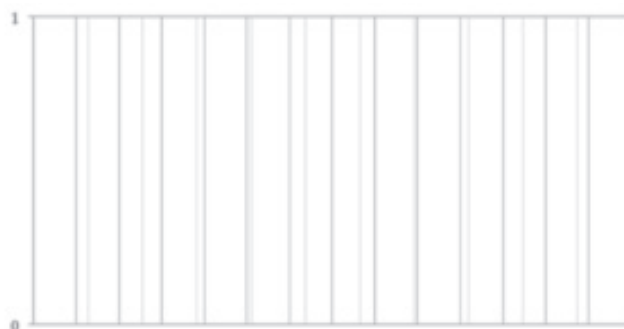
Figure 9: A spectral plot of two non-coincident impulse trains shows a more complex relationship. There is variability in the spacing between components and some clustering, leading to beating. The uniform magnitude of the components makes it very difficult to identify discrete pitches.
