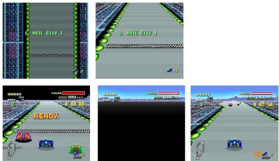
The composite image presented in Mode 7 in F-Zero . From top-left to bottom-right: 1) the natural view of the aerial 2D plane; 2) the deployment of Mode7 perspective effect by foreshortening the pixels at the top of the screen; 3) the 2D plane projected up to a horizon line, without the skyline background image; 4) the skyline image without the 2D plane projection; 5) the final, composite image with all layers.
